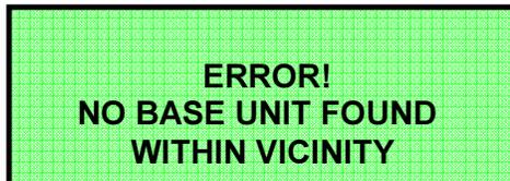
1. Check the power is switched on to the roller bed electronics.
