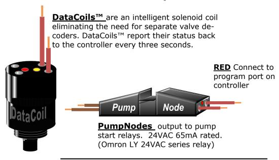
To program a DataValve or PumpNode number. Connect the valve or PumpNode to the **Two-**Wire Devices program port at the front panel of the controller, use the supplied leads.
