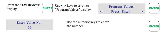
**Caution:** Ensure programming is correct before disconnecting from the program port. Once disconnected the device cannot be reprogrammed.
