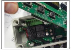
3. Attach power supply cable (ensure correct polarity).
