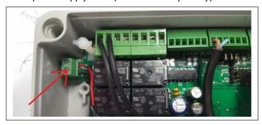
4. Attach pre-programmed DataNode (black wires).
